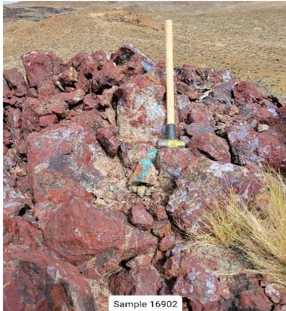
Photo 1 & 2: Red Hill outcrop, copper staining in brecciated jasperoids developed in rocks of the Candelaria formation. Sample 16902 reported 1.5% Cu over 1 meter.
